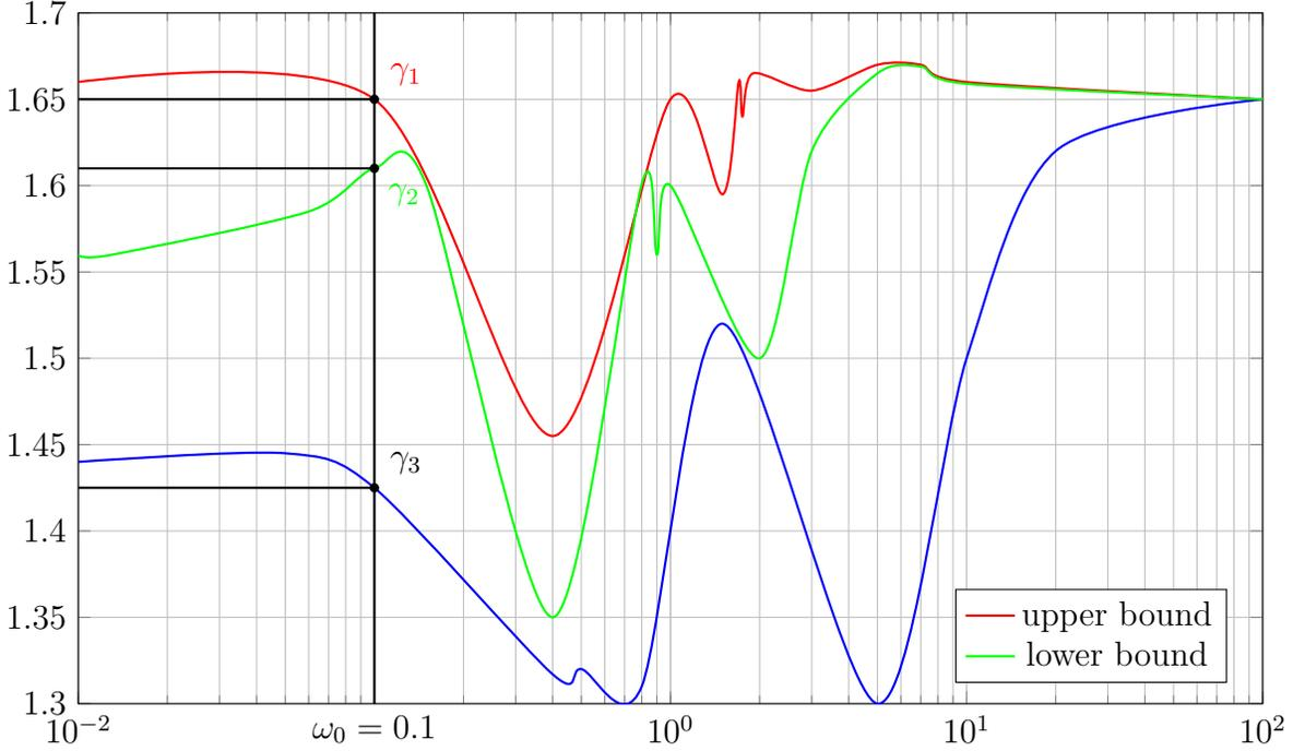
Figure 48: Plots of bounds on  $\mu_{\Delta_1}(M(i\omega))$  and of  $\rho(M(i\omega))$  over frequency.
