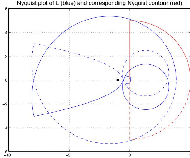
Figure 3: Nyquist plot of  $L$  for the satellite example. For the Nyquist contour we choose  $r = 0.1$  and  $R = 5$ .
