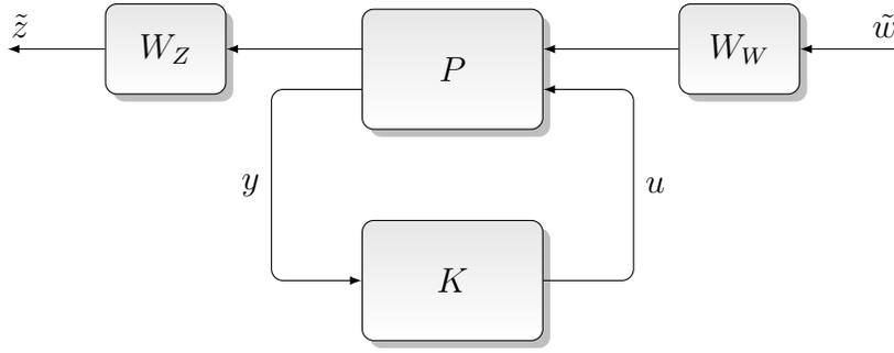
Figure 50: Weighted closed-loop interconnection
