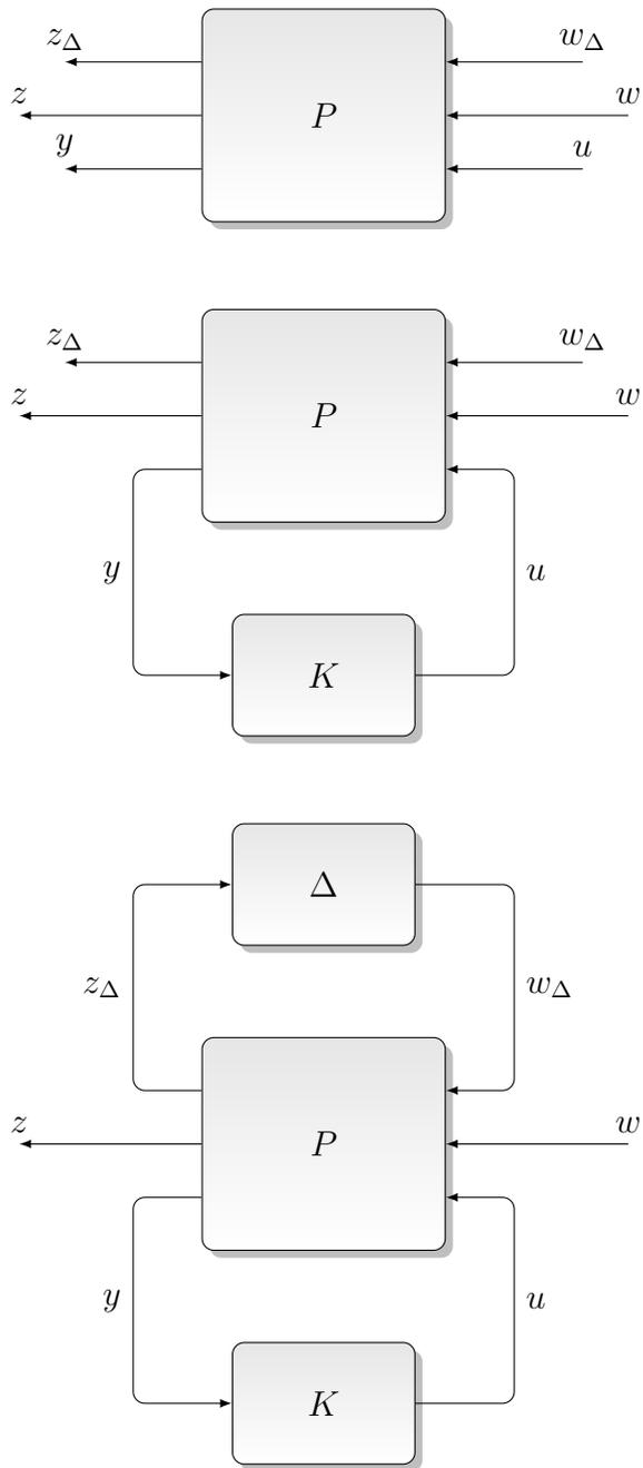
Figure 52: Open-loop interconnection, controlled interconnection, uncertain controlled interconnection.
