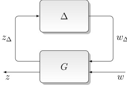
Figure 38: Uncertainty Pulled out of Component
