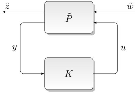
Figure 51: Weighted closed-loop interconnection
