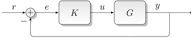
Figure 1: The standard tracking configuration.
