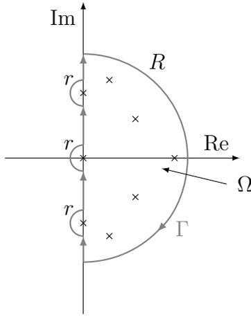
Figure 2: Nyquist contour  $\Gamma$  and encircled region  $\Omega$ ; crosses indicate poles of  $L$  in  $\mathbb{C}_= \cup \mathbb{C}_>$ .
