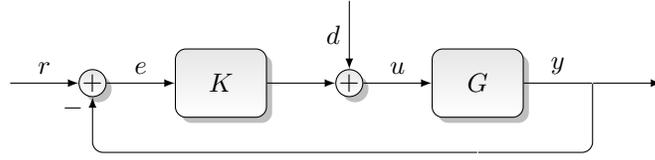
Figure 16: Standard tracking configuration with disturbance  $d$ .
