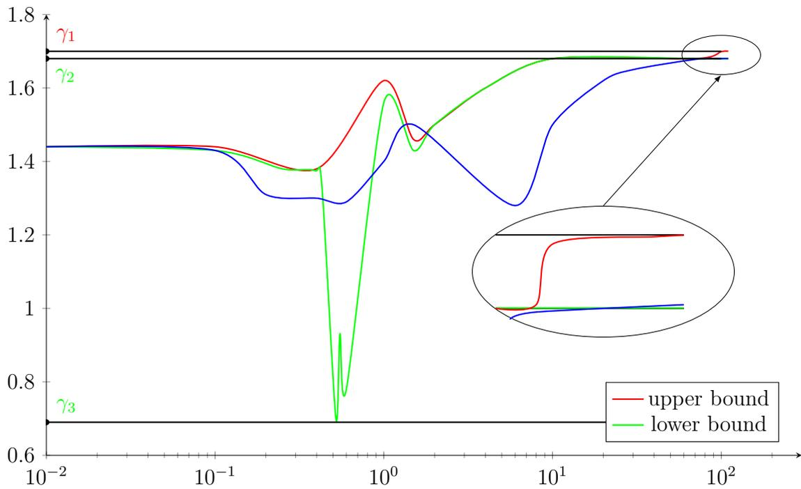
Figure 49: Plots of bounds on  $\mu_{\Delta_1}(M(i\omega))$  and of  $\rho(M(i\omega))$  over frequency.
