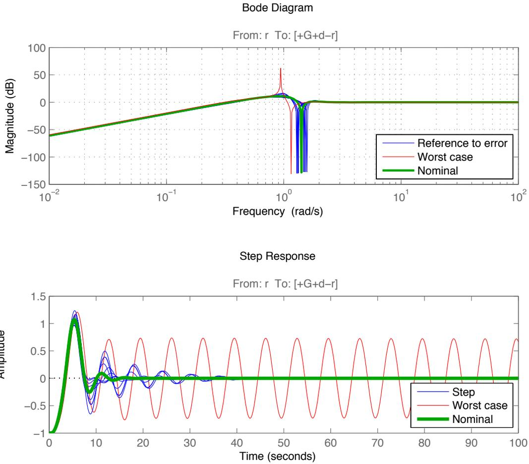
Figure 35: Samples of bode diagrams and step responses of a system affected by parametric uncertainties
