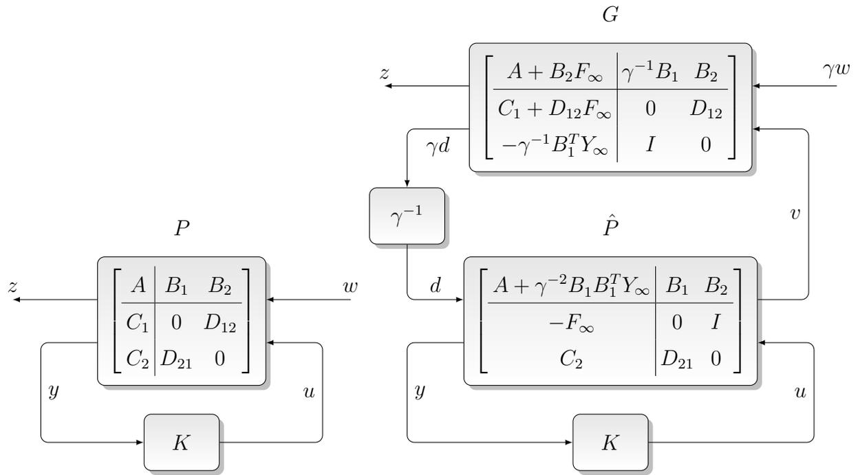
Figure 60: Re-description of the generalized plant  $P$ .
