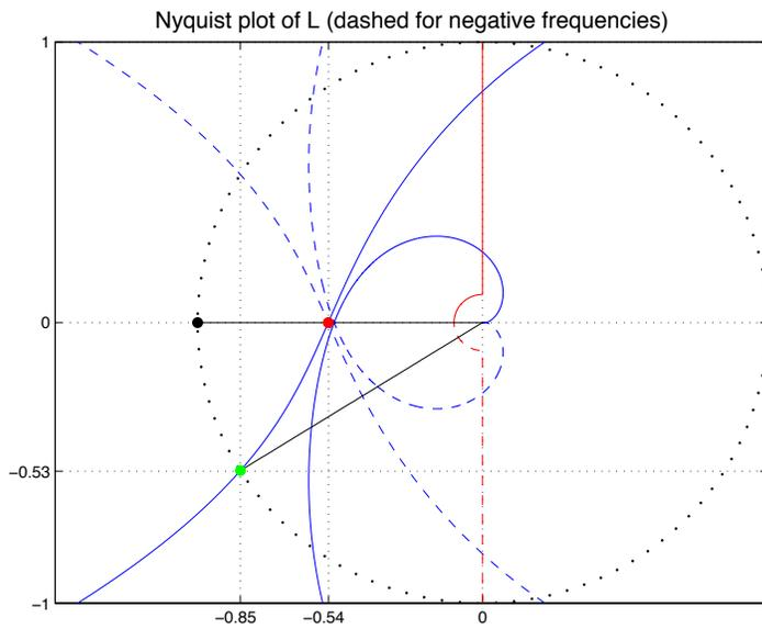
Figure 5: Nyquist plot with unit circle (dotted) and relevant crossing points.
