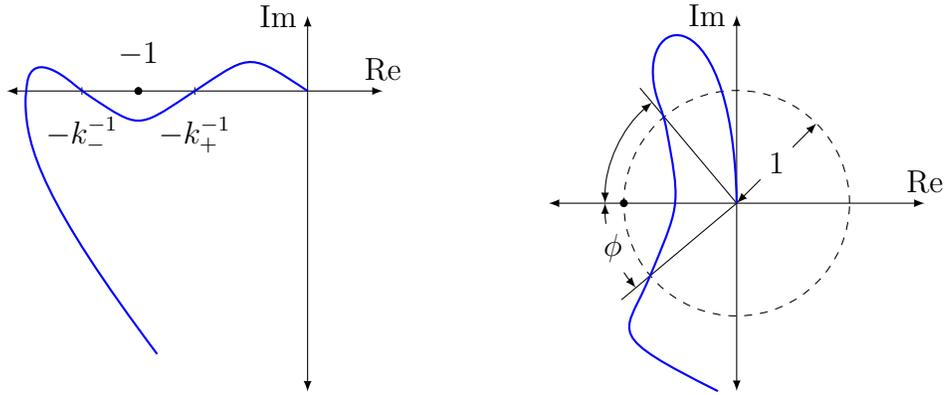
Figure 4: Graphical illustration of gain-margins and phase-margin.
