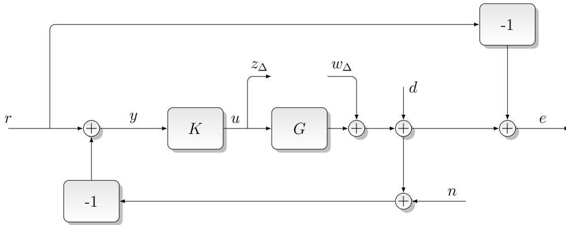
Figure 26: Closed-loop interconnection with disconnected uncertainty
