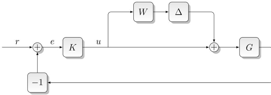
Figure 61: Tracking interconnection of simplified distillation column.
