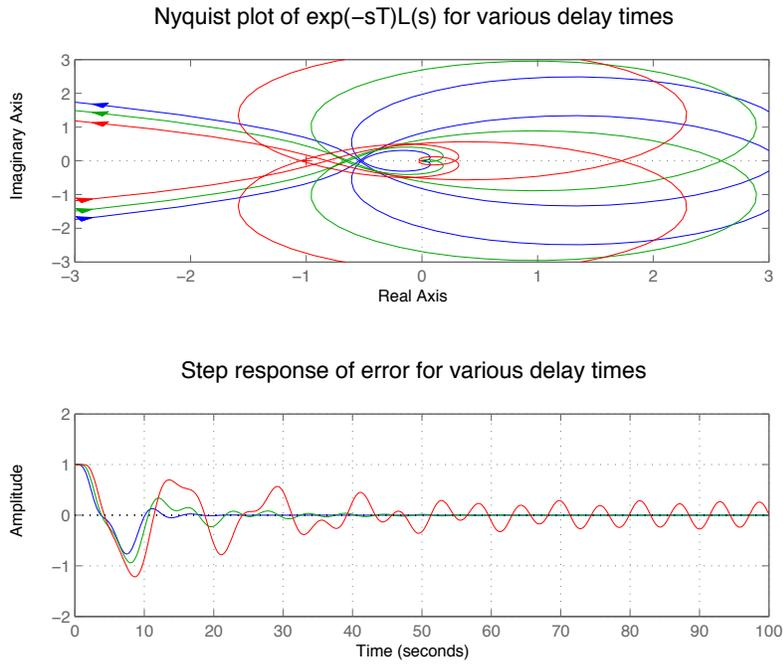
Figure 7: Responses of the system from Example 2.6 with time-delay  $T \in \{0, 0.4, 0.9\}$  in the loop.
