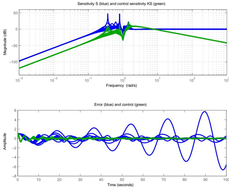
Figure 10: Samples of the Bode magnitude and step response.
