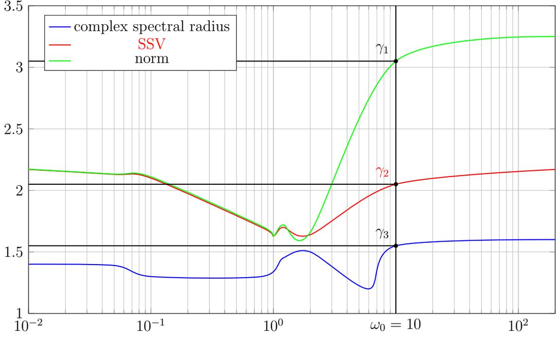
Figure 47: Plots of  $\|M(i\omega)\|$ ,  $\mu_{\Delta_1}(M(i\omega))$  and  $\rho(M(i\omega))$  over frequency.
