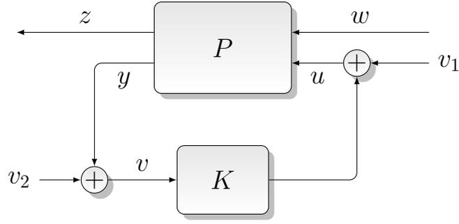
Figure 22: Interconnection to test whether  $K$  stabilizes  $P$ .
