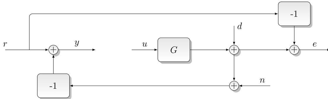
Figure 18: Open-loop interconnection that corresponds to Figure 17
