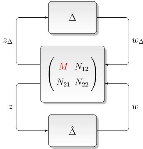
Figure 53: Equivalent Robust Stability Test
