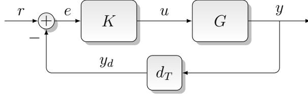
Figure 6: Standard tracking configuration with time-delay.
