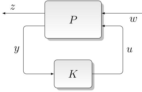
Figure 21: General closed-loop interconnection
